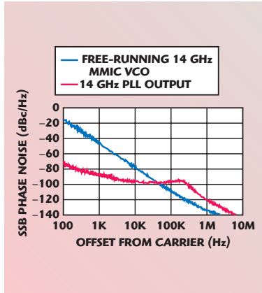
▲ Fig. 7 Measured phase noise .
